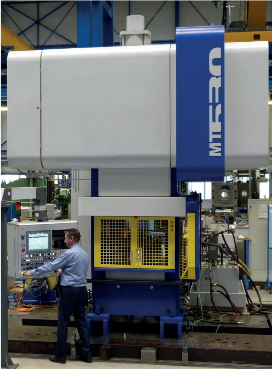
The Meertorque drive divides the eccentric drive into a coupled acceleration motor and a clutch-activated flywheel with its own motor. Photo: SMS Meer
