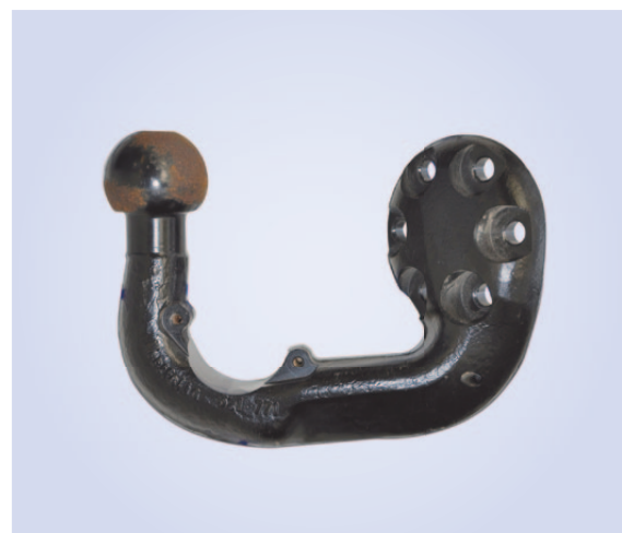
Figure 23: Ball head of the tow coupling
