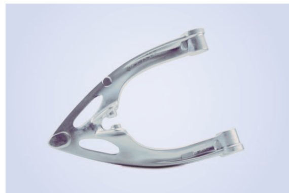
Figure 6: Motorcycle trailing link as an aluminium forging
