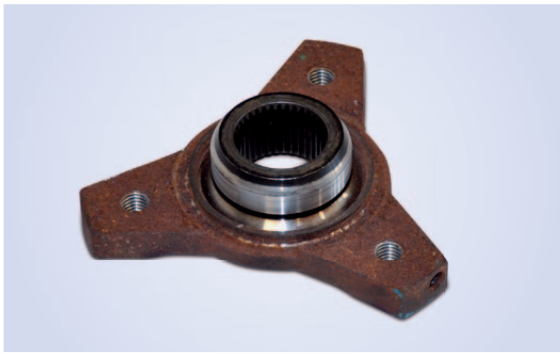
Figure 39: Companion flange of the drive shaft
