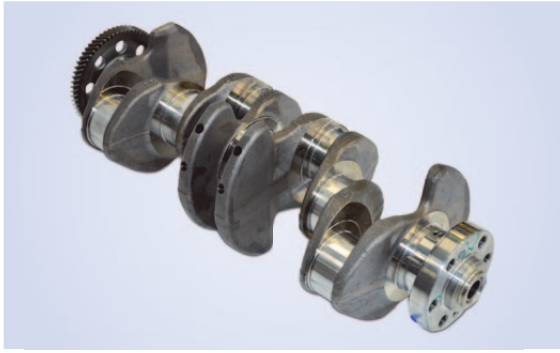
Figure 24: Crankshaft of the reference vehicle
