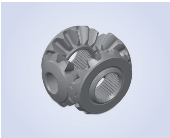
Figure 47: Optimized differential bevel gear set
