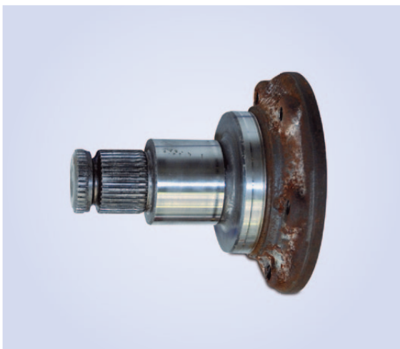
Figure 33: Companion flange input shaft – rear right
